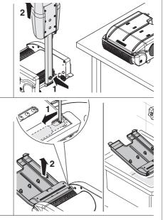
**3** Remove the brushes by pressing the button placed on the left side of the machine. Use a damp cloth to clean the internal sides of the machine while checking that seals are not clogged.
