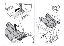
**4** Unhook and drain the clean water tank 2 from any residual of water and/or detergent.
