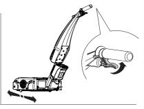
The engine of this appliance is equipped with a safety device which cuts it off in case of overload. If this situation occurs, it is necessary to return the handle to its initial position, turn off the battery and turn it on again, and then resume normal work. In the event that the engine does not work again, contact our after-sales service.
