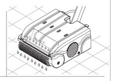
In the ongoing stage just pull the lever halfway; in the retuning stage, release the lever, thus allowing the liquid recovery.
