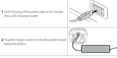
The correct charging of the battery will be signaled by the intermittent lighting of one of the LEDs positioned on the membrane and by the lighting of the red light on the charger.
