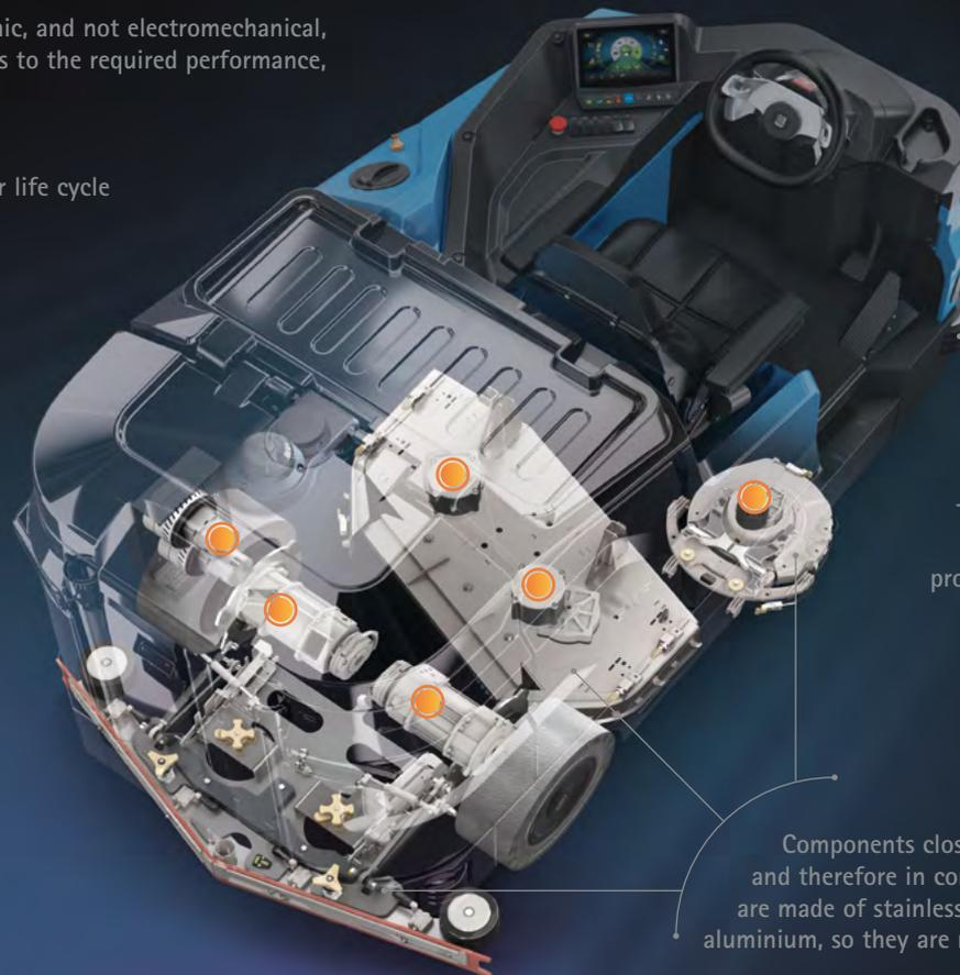
The roller bumpers at the 4 corners deflect shocks protecting the machine and extending its life
